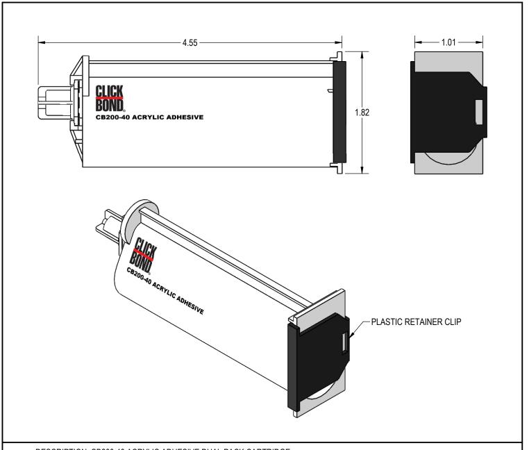
DESCRIPTION: CB200-40 ACRYLIC ADHESIVE DUAL PACK CARTRIDGE MATERIAL: ACRYLIC ADHESIVE, TWO PART, ROOM TEMPERATURE CURING CONTENTS: 40 ml ACRYLIC ADHESIVE, 2 PART, PRE-MEASURED
