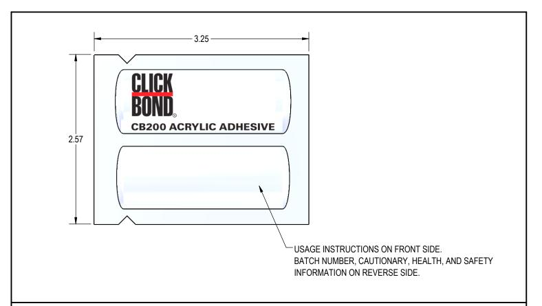
DESCRIPTION: FOIL PACKAGE CB200 ACRYLIC ADHESIVE, 2 PART, PRE-MEASURED, ROOM TEMPERATURE CURING QUANTITY: 3.5g
